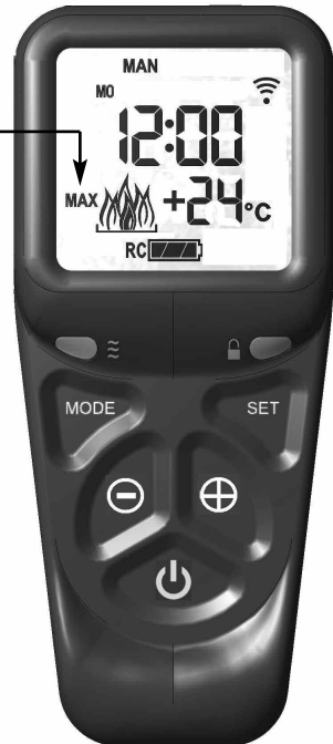
Fig. 26 - "MAX" & large flame symbol displayed
