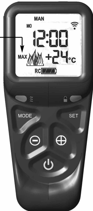
Fig. 3 - "MAX" & large flame symbol displayed
